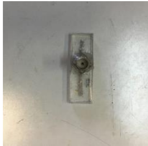
Figure 3. stretchable fabricated dipole antenna
