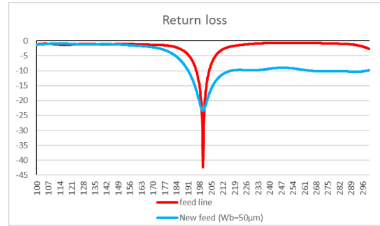
Figure 4. Return loss (dB), star patch antenna with feed line(blue) and new feed network(red)
