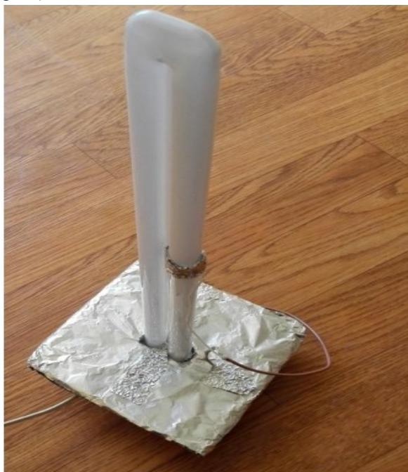
Figure 14. Fabricated folded monopole plasma antenna with sleeve coupling
