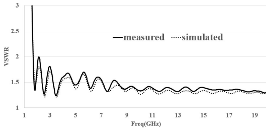
Fig 8. Compression between simulated and measured of VSWR
